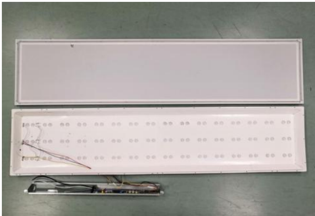
Photo 114 - Internal view for model BT.TW5S-1X4-NND-ZZ-YY-XXXX-RS
