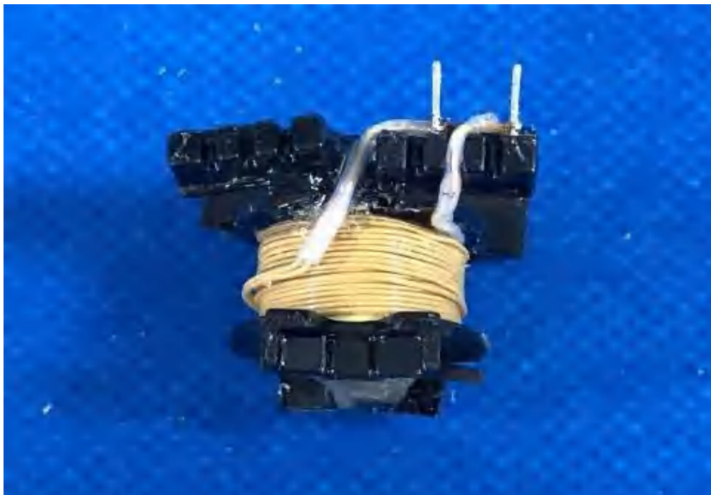
Photo 221a - Transformer (T1) construction of driver TR-031A
