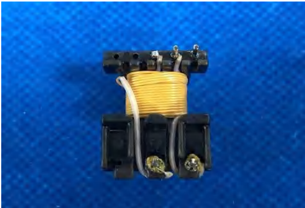
Photo 220a - Transformer (T1) construction of driver TR-019
