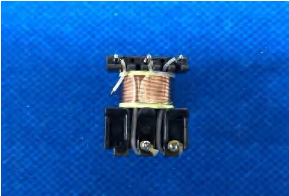
Photo 219a - Transformer (T1) construction of driver TR-120B
