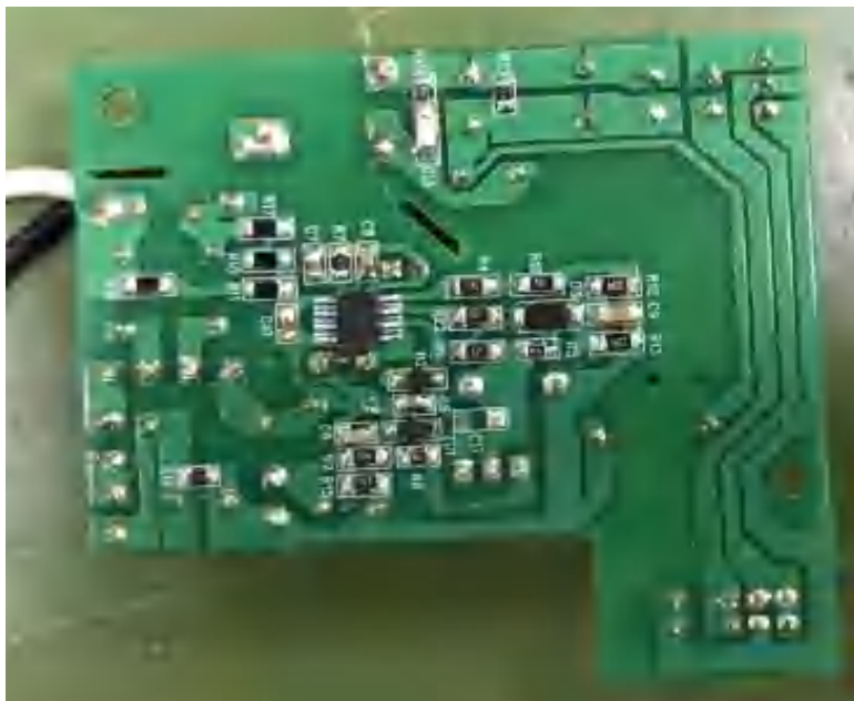
Photo 139 - Rear view of driver PCB of models JXL-TE06-T25W-CCT-xx, it also represent model JXL-TE08-T25W-CCT-xx
