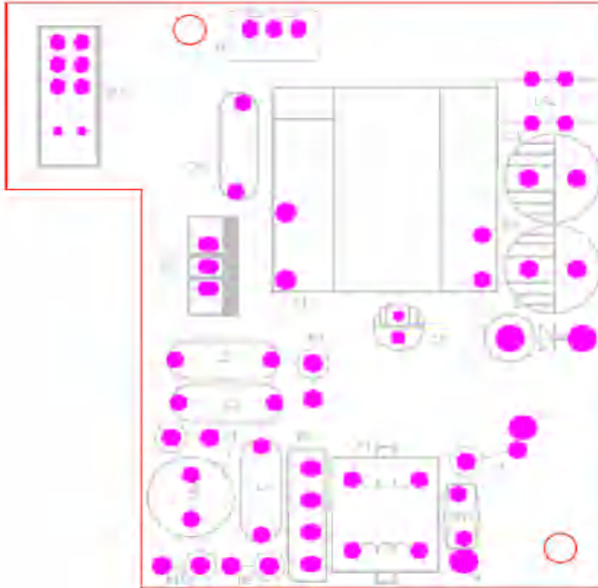
Illustration 28 - Top of PCB layout of driver of models JXL-TE06-T25W-CCT-xx, JXL-TE08-T25W-CCT-xx
