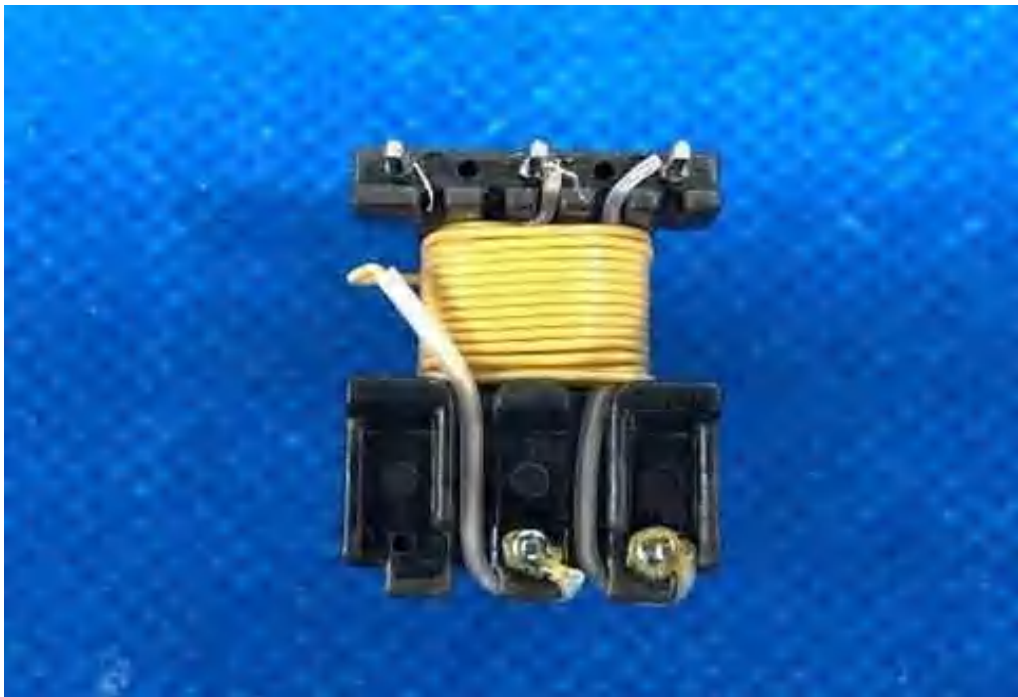
Photo 219a - Transformer (T1) construction of driver TR-120B
