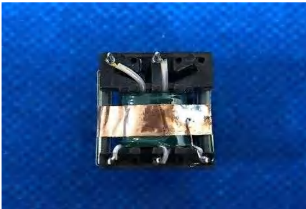
Photo 218 - Transformer (T1) construction of driver TR-120A
