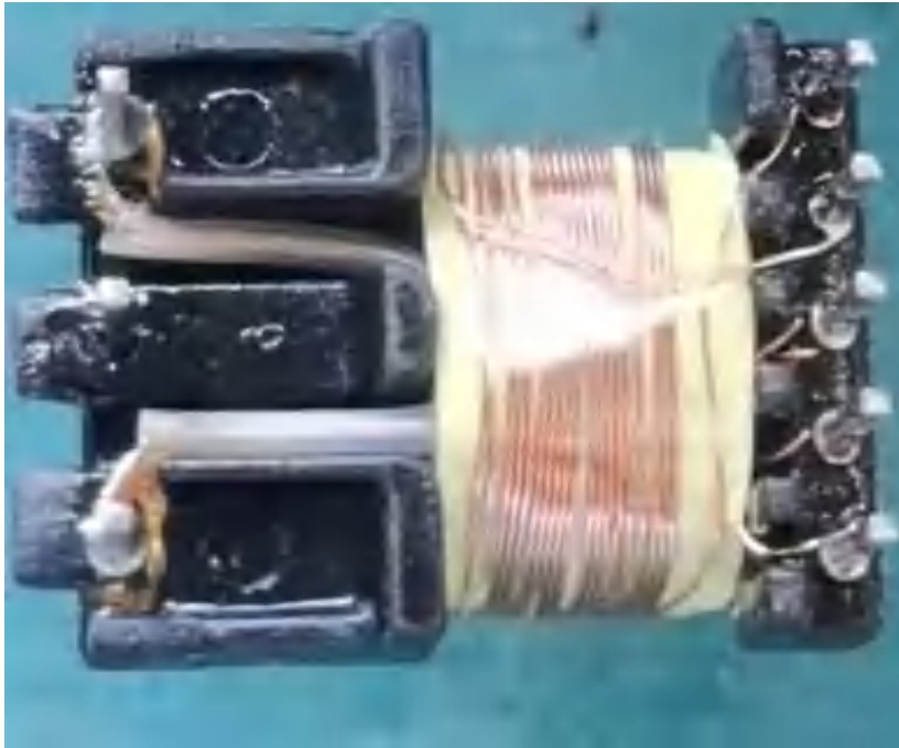
Photo 292- Transformer (T1) construction of driver TR-053 and TR-054
