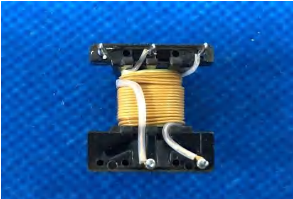
Photo 218b - Transformer (T1) construction of driver TR-120A
