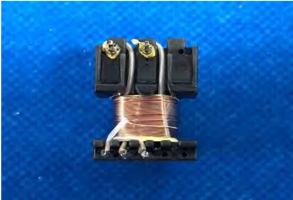
Photo 220a - Transformer (T1) construction of driver TR-019
