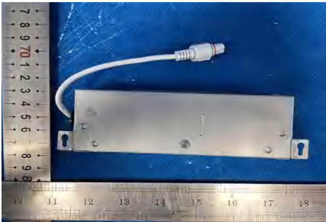
Photo 337 - External Bottom View of LED Driver TR-071
