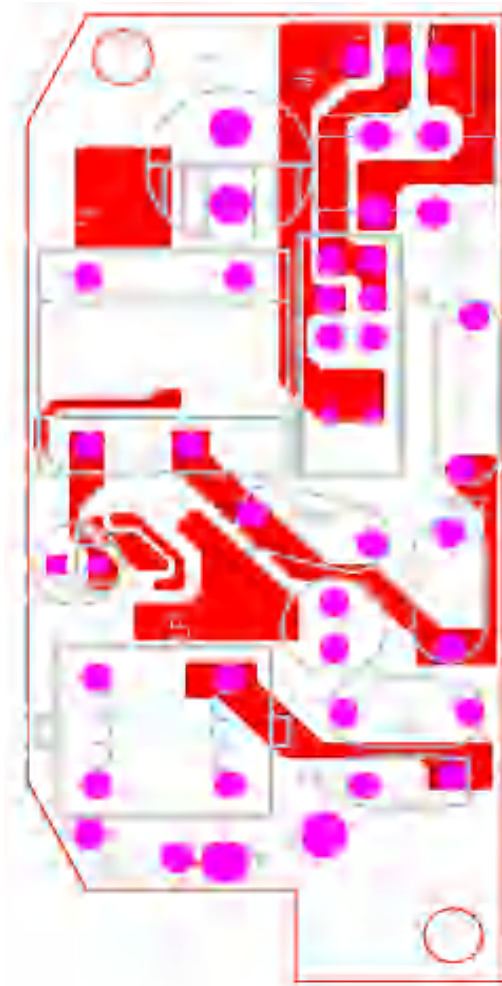
Illustration 8 - Top PCB layout of driver of models JXL-TZ04-T10W-CCT-xx and JXL-TZ06-T12W-CCT-xx
