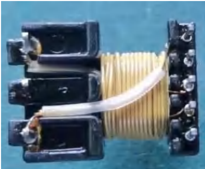
Photo 292- Transformer (T1) construction of driver TR-053 and TR-054
