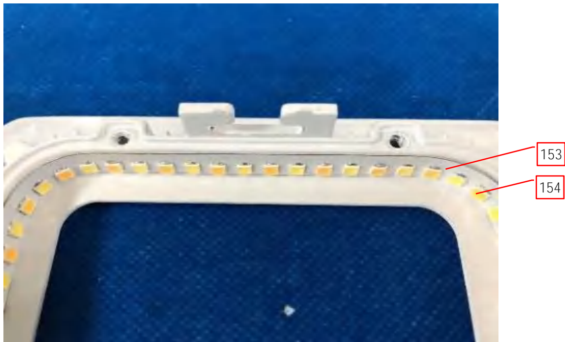
Photo 245 - Internal view of JXL-CF04-T10W-5CCT
