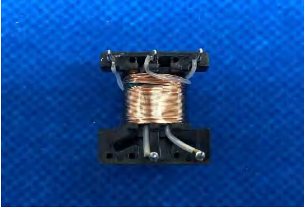
Photo 218a - Transformer (T1) construction of driver TR-120A
