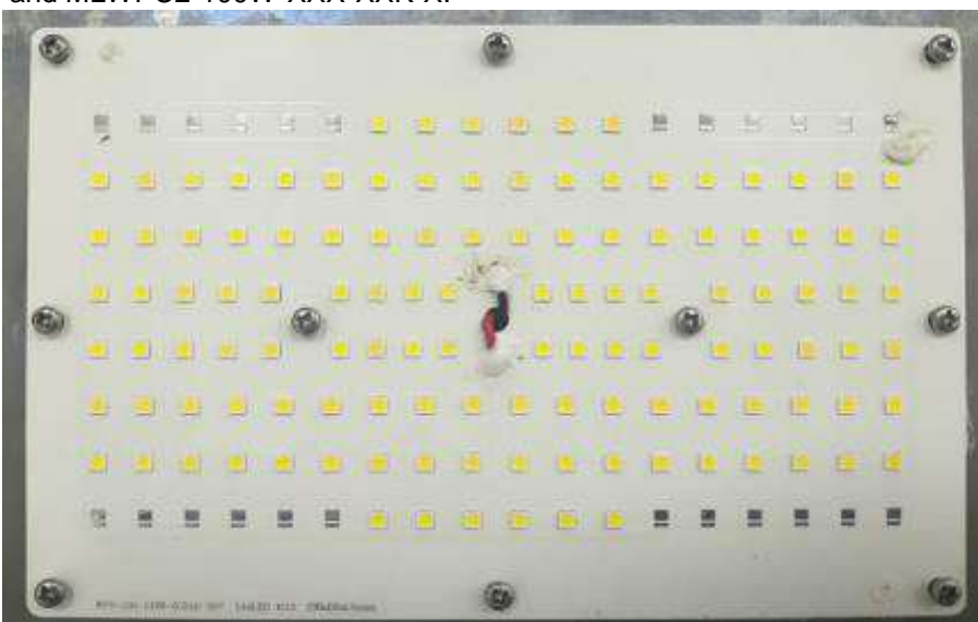
Photo 12 - LED PCB of MLWPB-100W-XXX-XXK-X
