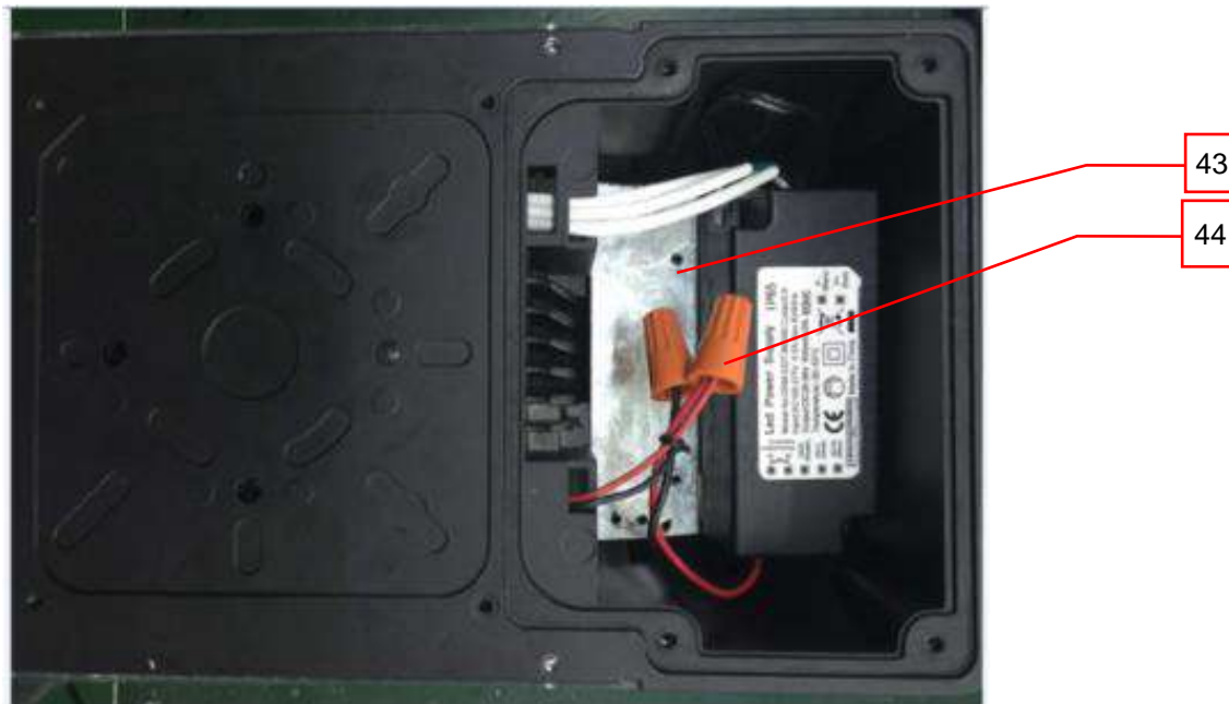
Photo 22 - Internal View of model ML-WPA-18W-XX, also represented model ML-WPA-26W-XX
