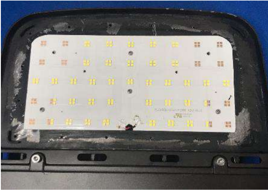
Photo 53 - LED PCB View of model PLC100WI-XXK-X, also represents series PLC models.
