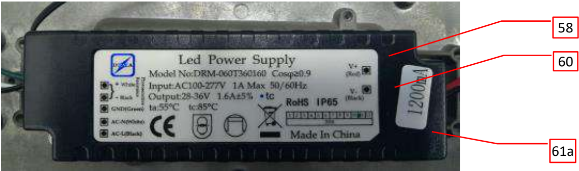
Photo 27 - Internal View of LED driver for DRM-060T360160-1 also represented DRM-060T360120-1
