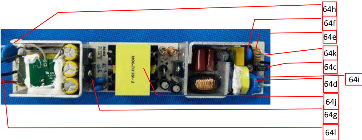
Photo 31 - Top View of PCB of LED Driver models ML-100T402300 also represented ML-080T40200, ML-120T402750
