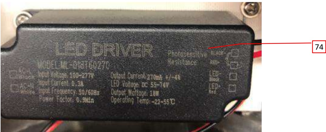
Photo 42 - Photo of LED driver ML-018T60270
