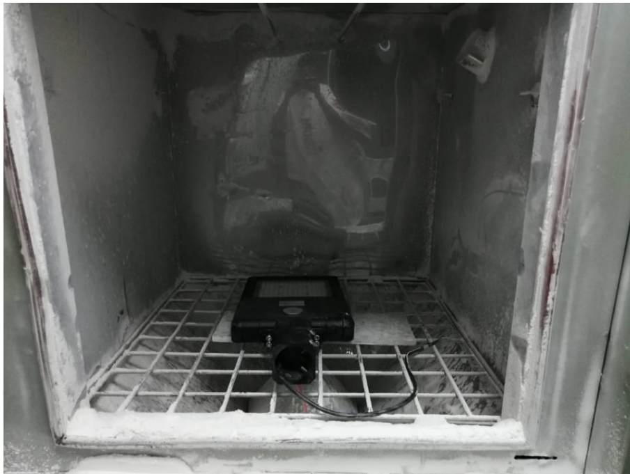
Photo 2: IP6X test of model AOK-120WoT-NV-L3-00-3070-T3-A
