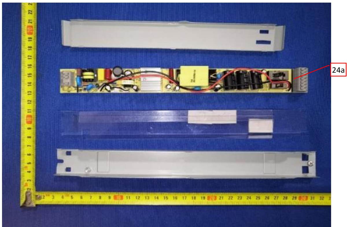
Photo 22 - Internal view of LED driver 2.
