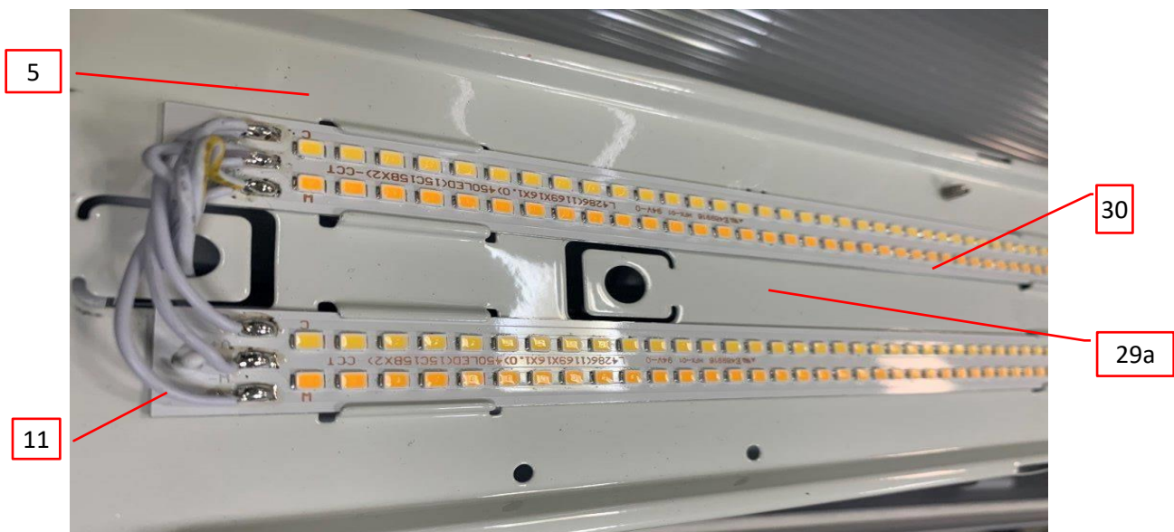
Photo 42a - LED PCB view of model TS-TPL3-8FT70W-X-TCP(MS) with alternative driver FS-TMG039B1520TCCP-12V and model TS-TPL3-8FT70W-X-TCP with alternative driver FS-TMG039B1520TCCP
