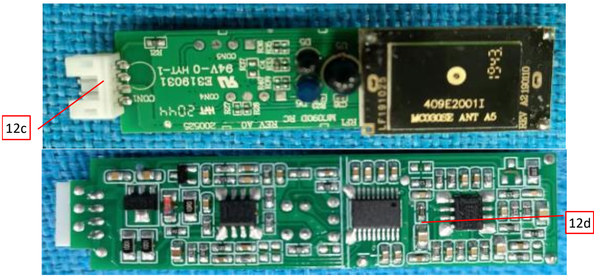
Photo 12a - Alternative Sensor PCB view of sensor model MC090D RC
