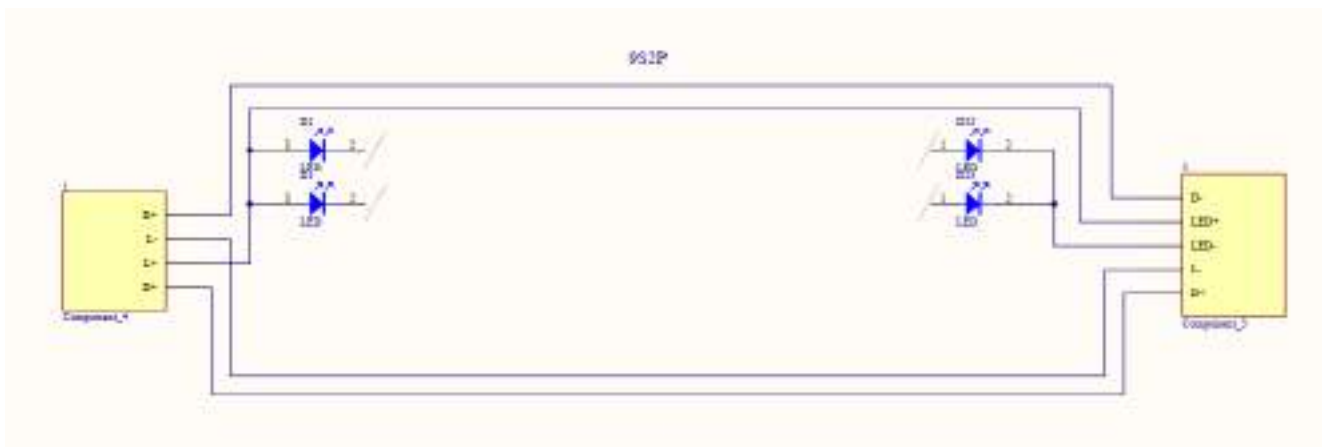
Illustration 59 - Schematic circuit diagram of LED PCB for model PVT8-24ND21-10W-%%-360-**K
