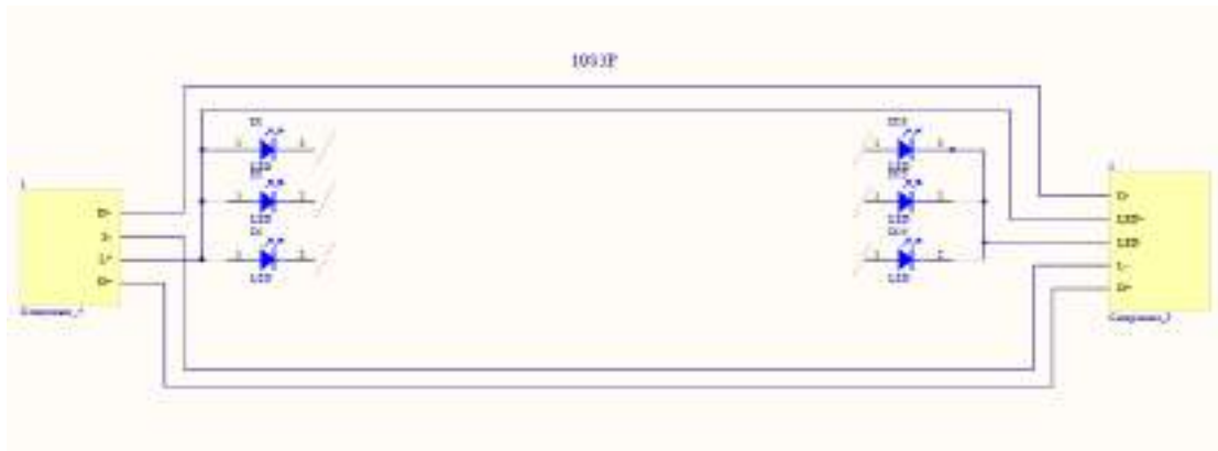
Illustration 62 - Schematic circuit diagram of LED PCB for model PVT8-42IND21-18W-%%-360-**K, PVT8-84IND21-37W-%%-360-**K.
