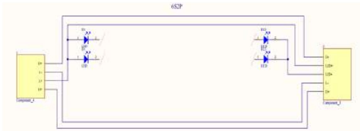
Illustration 58 - Schematic circuit diagram of LED PCB for model PVT8-18IND21-7W-%%-360-**K
