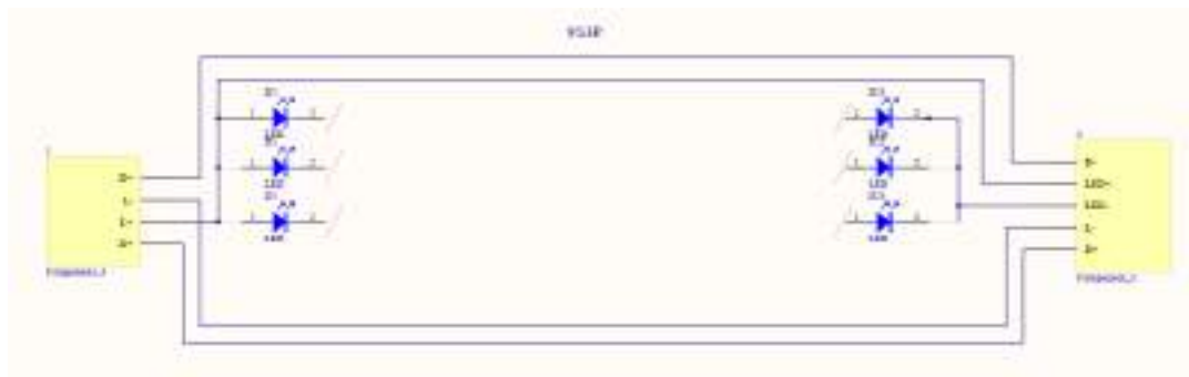
Illustration 61 - Schematic circuit diagram of LED PCB for model PVT8-36ND21-16W-%%-360-**K, PVT8-72IND21-31W-%%-360-**K.
